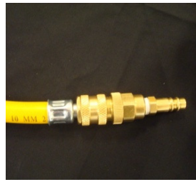
Step 1: Connect the Vetter air hose to the adapter.
