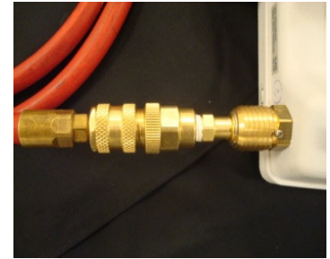
Step 2: Connect the Paratech air hose to the adapter.
