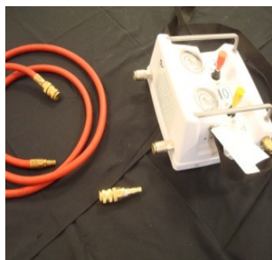
How to connect the Paratech air hose to the Vetter controller (air out)
