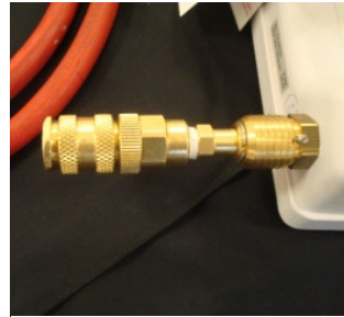
Step 1: Connect the adapter into the Vetter controller input
