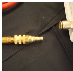
Step 1: Connect the Paratech air hose on the adapter.
