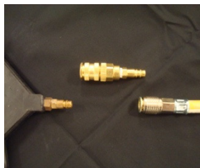
You need, Vetter air hose, Paratech air lifting bag and the adapter
