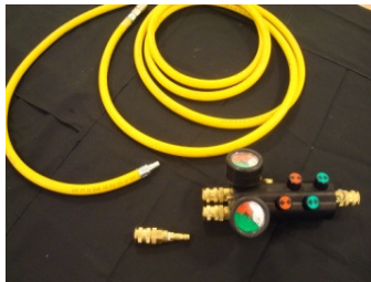
How to connect the Vetter air hose to the Paratech controller (air out)
