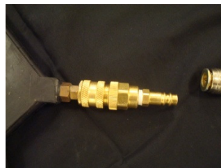
Step 1: Connect the adapter to the Paratech air lifting bag
