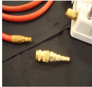
You need, Paratech air hose, Vetter controller and the adapter
