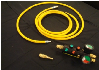
How to connect the Vetter air hose to the Paratech controller (air in)
