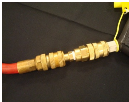
Step 3: Connect the adapter to the Paratech air hose
