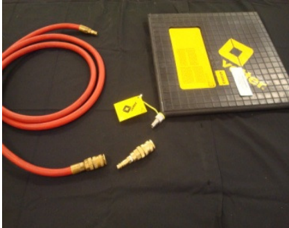
How to connect the Paratech air hose to the Vetter air lifting bag
