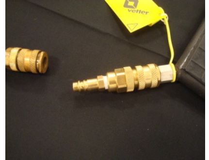
Step 1: Connect the adapter to the Vetter air lifting bag
