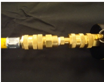
Step 3: Connect the adapter to the Paratech controller input
