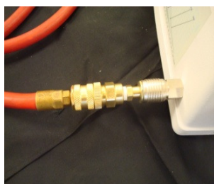
Step 3: Connect the adapter to the Vetter controller output
