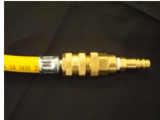
Step 1: Connect the Paratech air hose to the adapter.
