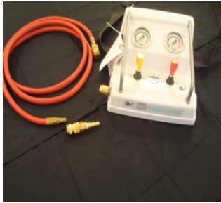
How to connect the Paratech air hose to the Vetter controller (air in)
